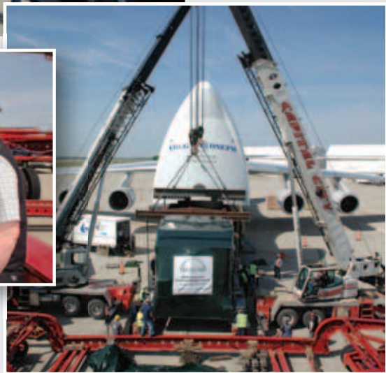
Diamond Heavy Haul, Inc. of Shandon, OH transported the turbine from the Rolls Royce plant in Mount Vernon, OH to the airport, using a Peterbuilt tractor and 2005 Diamond-built, 118 foot long, 11-axle 42-tire perimeter frame trailer
